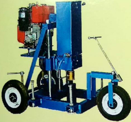
Core Drilling Machine Engine Type
