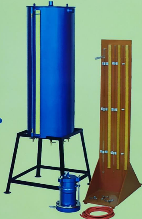
Soil Permeability Test
