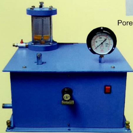
Dead Weight Type Oil & Water Constant Pressure System
